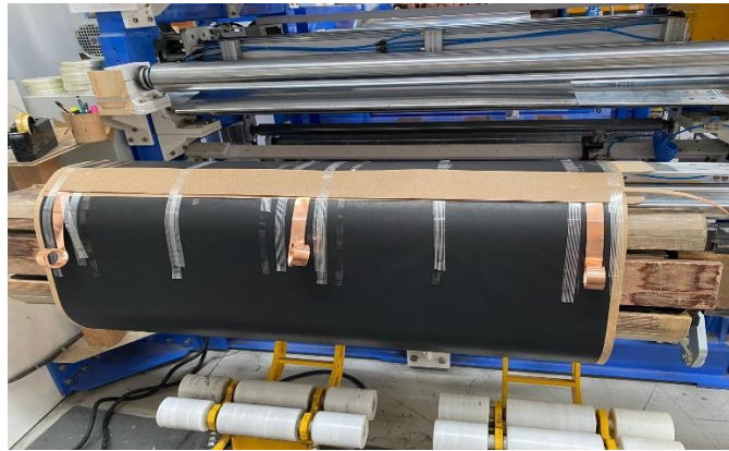
Fig. 18. The carbon loaded plastic shield used between LV & HV windings
